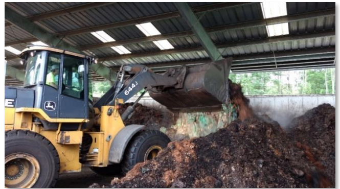
Figure 3. Blending (each time food waste is delivered)
